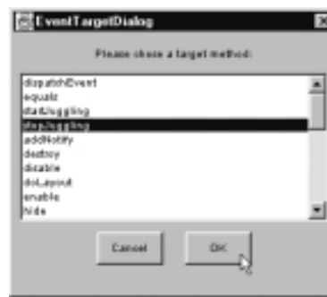
Fig. 25.13 The EventTargetDialog window displays the list of methods that can be called on the target of an event.
